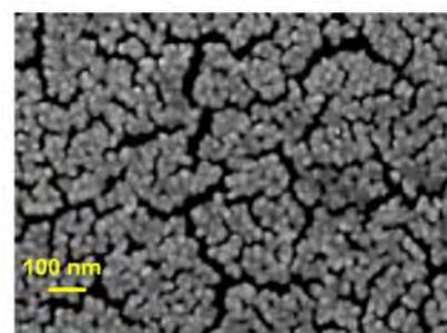
Fig.2 SEM image of silver nanoparticles on sample surface.
