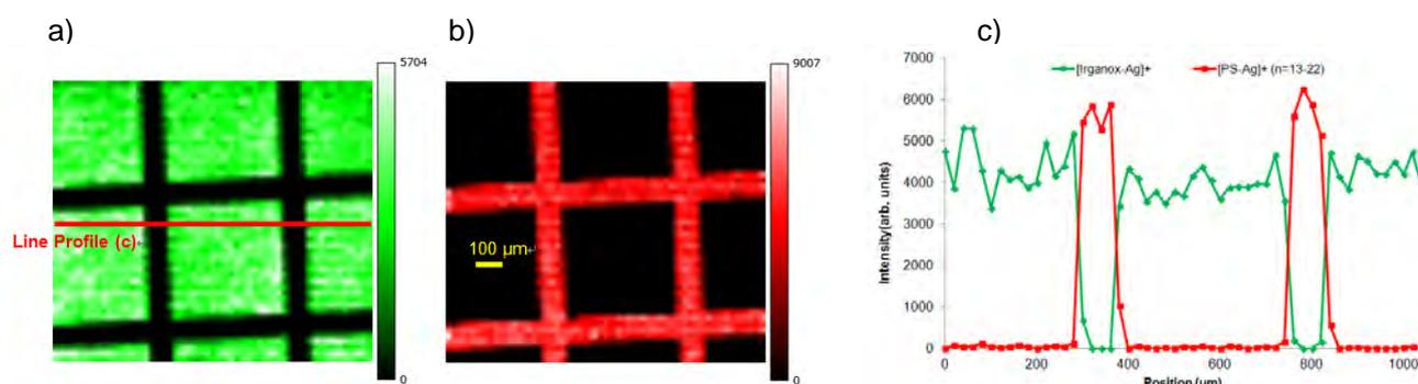
Fig.4 Ag-NP SALDI IMS for Irganox 1010 on PS layer.
