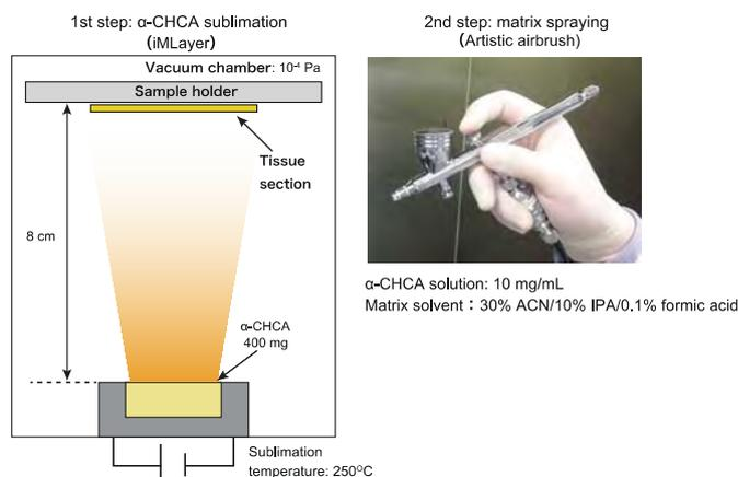
Figure 1 Workflow of two step matrix application method.
