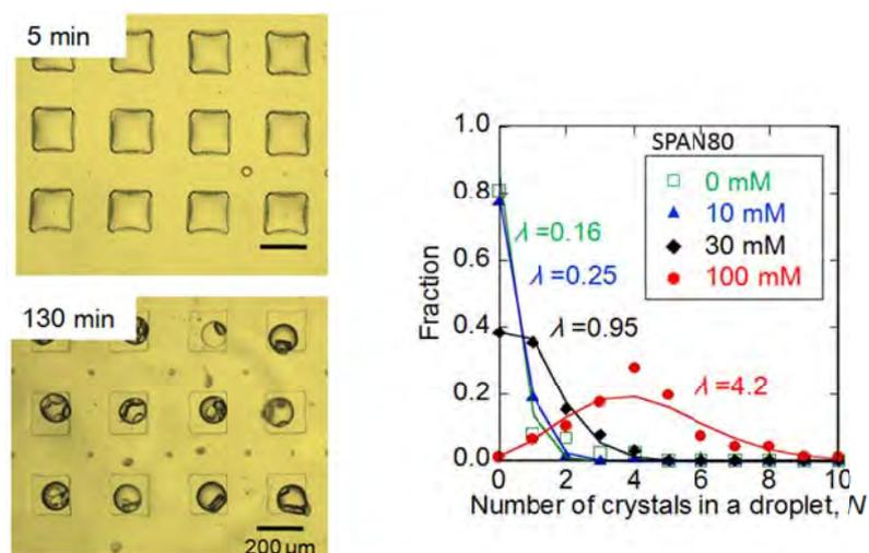
Figure 4 Microwell-based droplet formation and protein (lysozyme) crystallization utilizing spontaneous emulsification. The number of crystals in a droplet depends on the condensation rate, which can be controlled by the surfactant concentration. [4]
