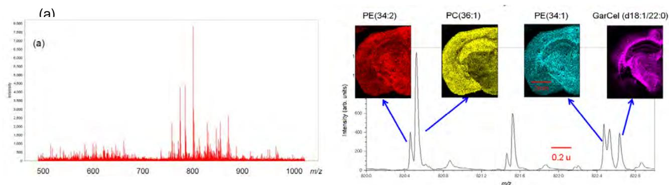
Fig.3 High mass resolution IMS for lipids in brain tissue section.
