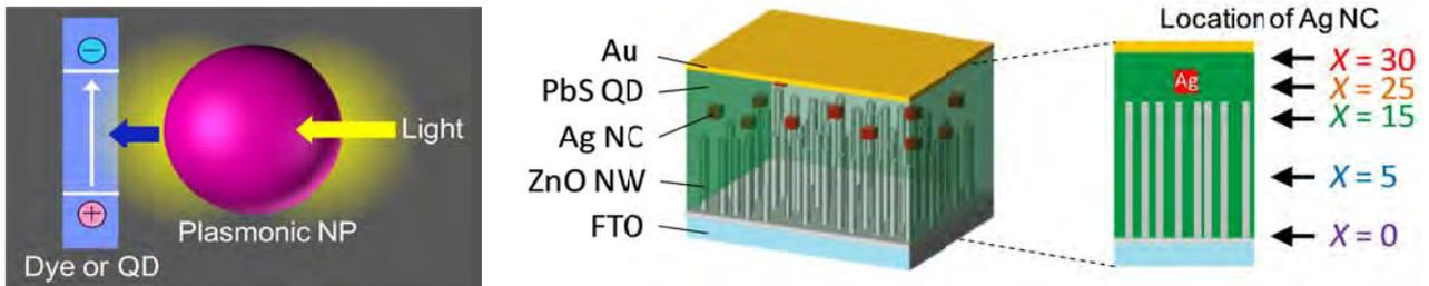
Plasmonic nanoantenna effect. Colloidal quantum-dot solar cell with plasmonic nanoantennae.<sup>5</sup>
