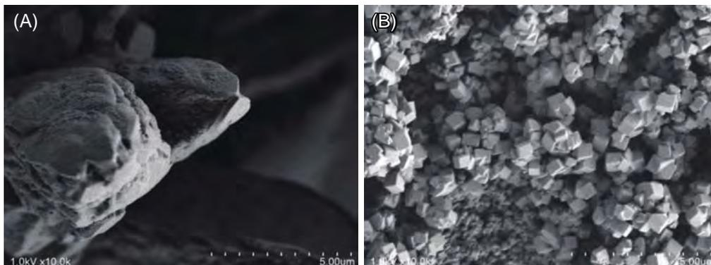
Figure 2 Difference of  $\alpha$ -CHCA crystal morphology between conventional spraying and two-step method. (A) Conventional and (B) two-step method. (Magnification of 10k).
