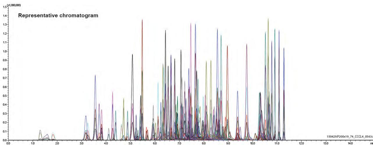
Analysis of over 200 pesticides residues in cannabis using triple quadrupole LC-MS/MS.
