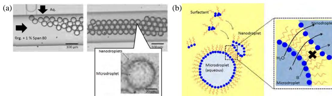
Figure 1 (a) Aqueous microdroplet formation in organic phase with surfactant (Span 80) (left), and spontaneous emulsification on the microdroplets (right). (b) Conception of selective enrichment of solute during the spontaneous emulsification. [2]
