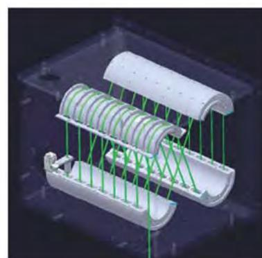
Fig.1 Spiral ion optical system
