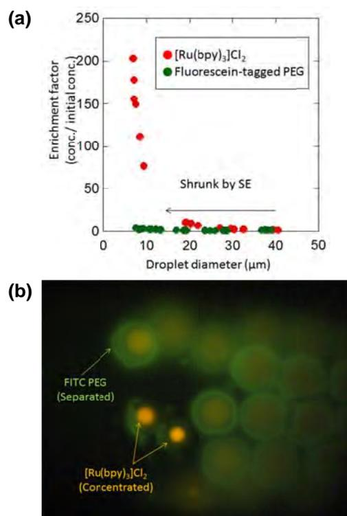
Figure 2 (a) Enrichment factor during spontaneous emulsification. (b) Micrograph of selective enrichment. [2]
