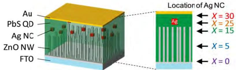
Colloidal quantum-dot solar cell with plasmonic nanoantennae.<sup>5</sup>
